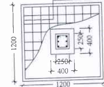
DETAILS OF R. C. C COLUMN (SCALE - 1:25)
