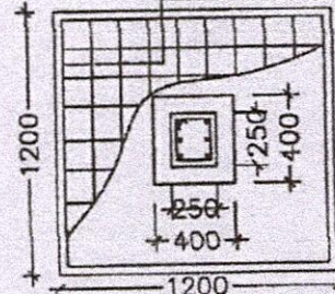
DETAILS OF R. C. C COLUMN (SCALE - 1 : 25)
