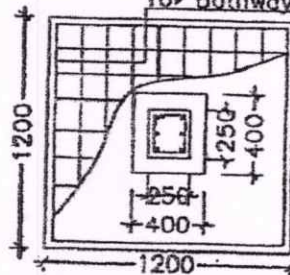
DETAILS OF R. C. C COLUMN (SCALE - 1 : 25)
