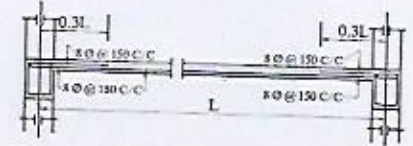
Details Of R.C.C Roof Slab & Beam (SCALE - 1:25)
