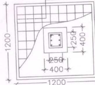
DETAILS OF R. C. C COLUMN (SCALE - 1 : 25)
